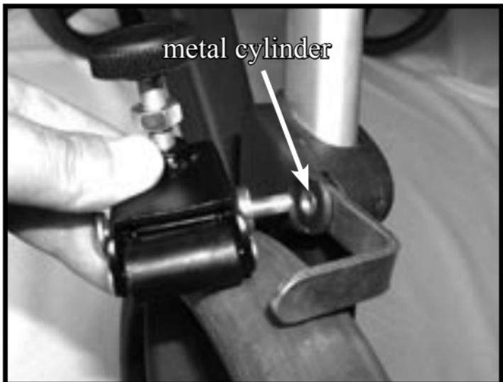
Step 3: Tighten screw firmly, but do not overtighten (brakes must function).
